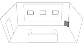
The spacing of the left-right speakers can be a little wider than with 2-channel stereo speakers, since in a theater system, the center channel speaker reproduces the on-screen effects and anchors the center image. Left-right spacing of about 8 to 10 feet usually works well.
