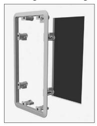
The clamping mechanism allows the wall material to range from ½ to 1½ inches (13 to 38 mm) in thickness. There must be a minimum depth behind the wall face of 3 5%" (92 mm). As noted above, be sure to keep the edges of the cutout at least ½ inch (13 mm) away from any stud or obstruction, as the rotating clamps will not operate properly if you don't. Insert the frame into the cutout and using a level or square carefully align it so it is level. Tighten the mounting screws, which will
