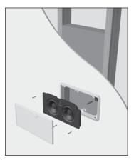
For new construction, we highly recommend that you use the optional Back Box IN-BOX-155. The Back Box provides the correct acoustic environment for the 155 LCR and ensures its THX-level performance. The rotator clamps (sometimes called "dog legs") will easily grab the combined thickness of 5/8" sheetrock and the 3/8" back box's front panel. The sheetrock must be adhered to the front panel of the back box very solidly and positively.
