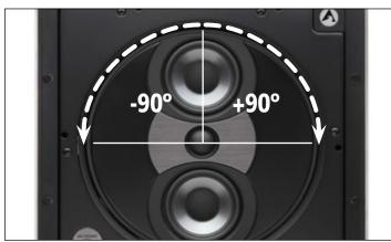
M-T-M baffle can be rotated 90 degrees from center. Do not exceed this rotation angle to avoid putting undue stress on the midrange-tweeter lead wires.
