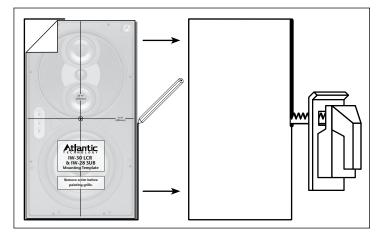
After determining the best location for the speaker as outlined above, use the enclosed template to cut the proper size hole.
