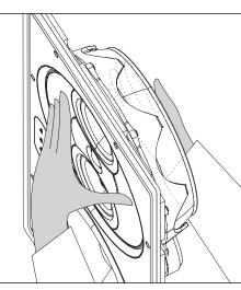
To rotate the baffle, hold the baffle on the front and rear flat surfaces (being careful not to press on the midrange or tweeter diaphragms) and turn the M-T-M baffle to its desired position. Do not exceed 90° of rotation to avoid putting undue stress on the midrange-tweeter lead wires.
