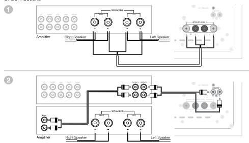
Disconnect all audio system equipment from the mains until the signal connections have been made and checked. This avoids the risk of damage whilst connections are made or broken. The subwoofer can accept both line level signals via the RCA Phono sockets and speaker level signals via the binding posts.
