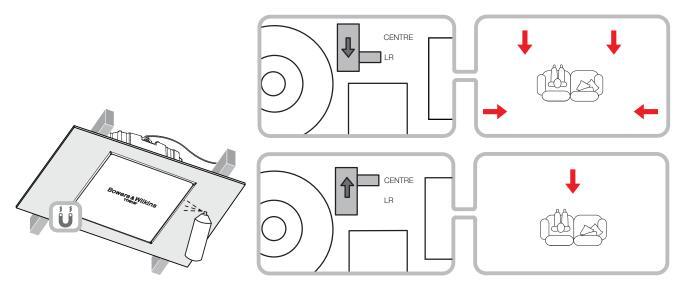
4.6 If the back box flange is to be painted it should be done at this stage. Any conventional, domestic paint may be applied by brushing, rolling or spraying. Use the supplied paint mask to avoid getting paint in the back box cavity. Painting without using the paint mask risks contamination of the internal connection terminals or the grille attachment magnets. The diagram above illustrates painting using the paint mask.
