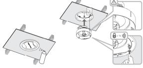
4.5 If the frame flange is to be painted it should be done at this stape, Any conventional, domestic paint may be applied by brushing, rolling or spreying. Use the supplied paint mask to avoid getting paint in the cavity. Painting without using the paint mask risks contamination of the internal connection terminals or the grille attachment magnets. The diagram above illustrates painting using the paint mask.
