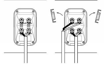
Ensure that the positive terminals on the speaker (marked + and coloured red) are connected to the positive output terminal on the amplifier and the negative terminals on the speaker (marked – and coloured black) are connected to the negative output terminal on the amplifier. Incorrect connection can result in poor imaging and loss of bass.
