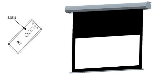
Press the **16:9** button on the RF remote, this will retract the 2.35:1 screen into the housing. When the 2.35:1 screen has stopped, the 16:9 screen commences its deployment.
