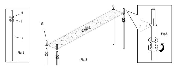
5. Lastly, align the end flange holes to the threaded support rods and fasten them with the nuts and washers as show below.
