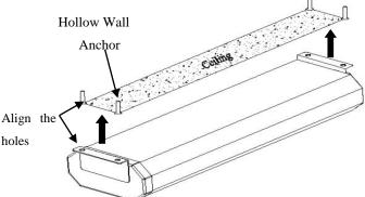
4. Insert the *screw* (B) in the *hollow wall anchor* (A) and fasten with a *screw* (B) to secure the screen in place. Repeat procedure until screen is safely installed.
