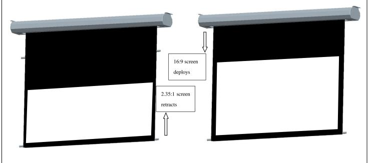
Press "UP" button on the RF remote to retract the screen into the housing.
