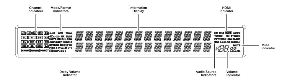
**Channel Indicators:** These will light to show which channels are active based on the input format and processing that is selected. Note that the indicators respond to the audio format and processing that is selected and audio will not be present from a channel at all times even when they are illuminated.
