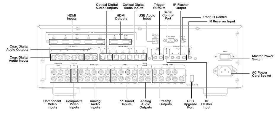
HDMI Inputs: Connect the output of an HDMI source device to these jacks.
