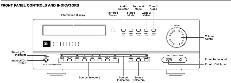
**Standby/On Indicator:** This LED indicator will light red when the AC mains power is applied and the rear panel Master Power Switch is turned on. It will turn blue when the unit is turned on from the front panel Standby/On Switch, the remote control or an external control system.
