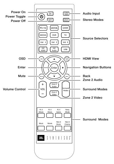
Power Toggle: Press this button to turn the unit on or place it in the Standby Mode.
