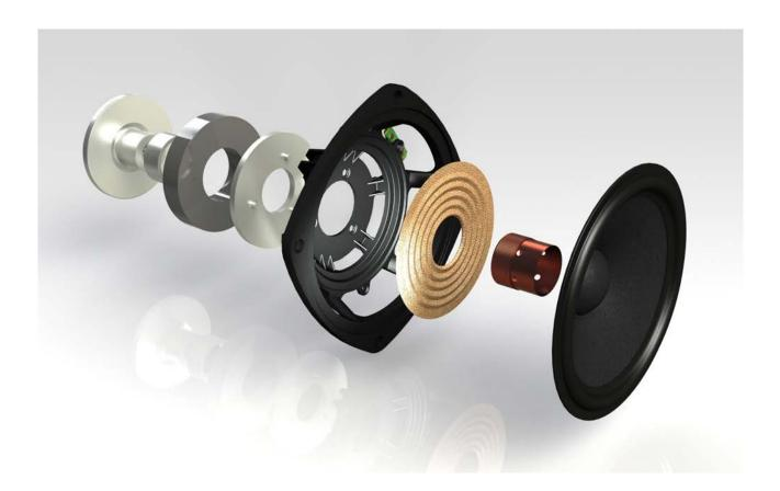
**5.** Miller & Kreisel custom made aluminum basket employs open frame (7 mm flange) with rigid rib structure for mechanical stability and full ventilation under the spider and cone to eliminate power compression and drastically reduce 3rd harmonic distortion.
