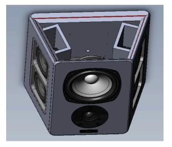
The dual sets of side-firing drivers 4 inch. incorporate a small network to ensure that the side drivers closest to the front tweeter do not interfere with the dispersion of the front firing tweeter.
