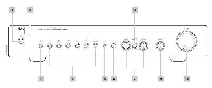
STANDBY: With the rear panel POWER switch set to ON position, press this button to switch ON the C 316BEE from standby mode. The Standby LED indicator will turn from amber to blue. Pressing the STANDBY button again turns the unit back to standby mode.
