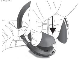
**2** Fit the ear cup to the ear pad until the magnets snap them together. Ensure fit for form and no misalignment.
