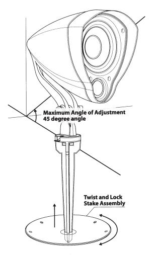
extreme temperatures, the loudspeaker should not be placed at an angle greater than 45° above a horizontal position in order to prevent the possibility of excessive amounts of water staying within the top housing and freezing in cold environments, which could damage the loudspeaker.
