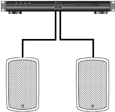
Figure 3. Wiring directly from a receiver or amplifier
