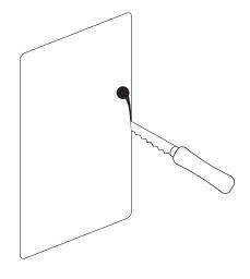
**NOTE:** Before cutting the speaker opening, be sure to cut carefully to make the opening as symmetrical as possible. However, with the speaker in place, it will overlap some of the cutting edge, which will mask minor cutting inaccuracies.
