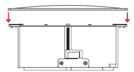
III. If the grille will not lock into place, check to ensure the grille is properly centred on the frame, and all magnets are clear of all debris and material for proper installation.
