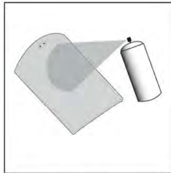
FIGURE 9: Paint the grille. Use thin coats of spray paint. Do not block grille holes with paint.
