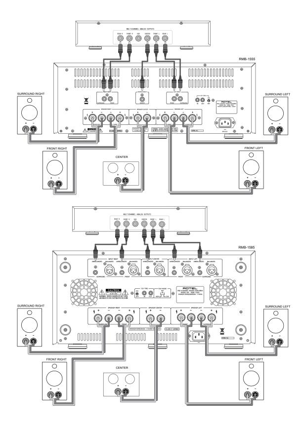
Figure 3: Balanced (XLR) Inputs
