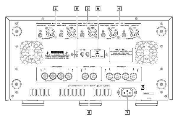
Figure 2: Analog Inputs and Speaker Output Connections
