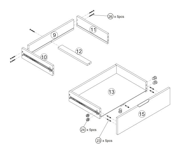
When inserting cam, ensure arrowhead on cam points toward to the hole on the panel edge.
