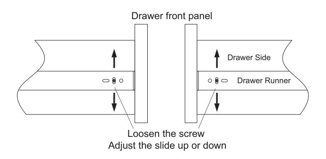
Loosen the screws on the left and right hand side, then move the drawer slide up or down, untill the drawer fronts are even/level, then tighten the screws
