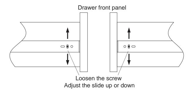
Loosen the screws on the left and right hand side, then move the drawer slide up or down, untill the drawer fronts are even/level, then tighten the screws
