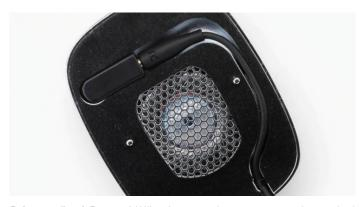
**Drivers refined** Bowers & Wilkins' renowned engineering team has worked wonders on P3 Series 2's small drive units. They have redesigned the driver to include a unique damping system to control diaphragm movement for improved resolution.
