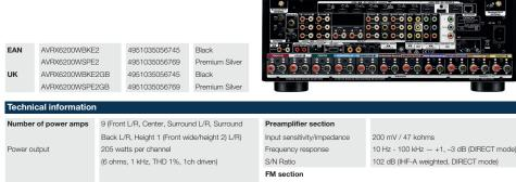
87.5 - 108 MHz 175 watts per channel Tuning frequency range (6 ohms, 1 kHz, THD 0.7%, 2ch driven) AM section 522 kHz – 1611 kHz Tuning frequency range 140 watts per channel General (8 ohms, 20Hz - 20 kHz, THD 0.05%, 2ch driven) Power supply AC 230 V, 50/60Hz Power consumption 730 W (Standby 0.1 W, CEC standby 0.5 W) 4 - 16 ohms Power consumption No-Sound 65 W (ECO on), 110 W (ECO off)
