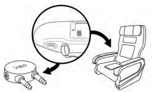
Use the supplied dual 3.5mm airline adaptor to connect your VISO HP30 with in-flight entertainment systems.
